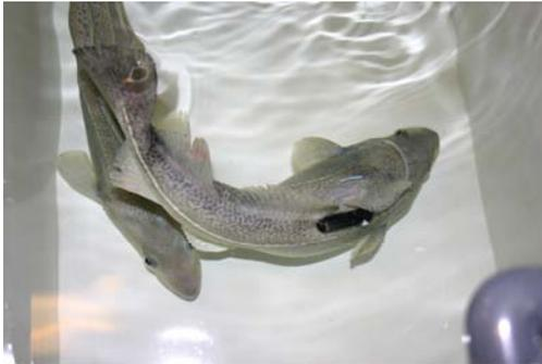
*The SmartTag (46 x 16 mm, 6 / 15 g in water/air) is attached on the back of the anaesthetized fish.*
