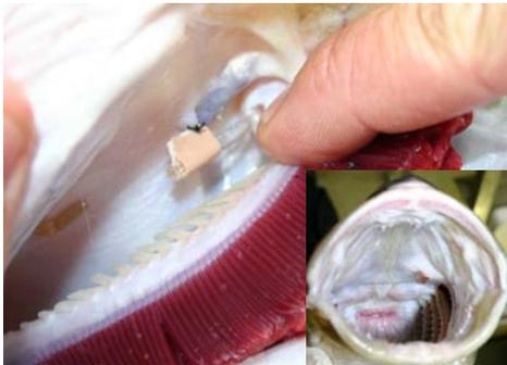
*A 1.6 mm ID tube inside the mouth and connected to the tag provide online pressure measurements, thus producing detailed data on fish breathing activity.*
