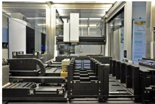
Robotic platform with high-throughput liquid handler for sample preparation , dilution and test-plate treatment. Supported by optical plate reader , plate washer and incubator
