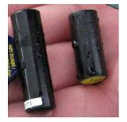
Acoustic and dataloggers - used in FW & SW
